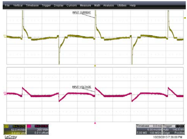
Figure 62 – 45° Conduction Angle. Upper: I_{IN} , 50 mA / div. Lower: V_{IN} , 200 V, 5 ms / div.
