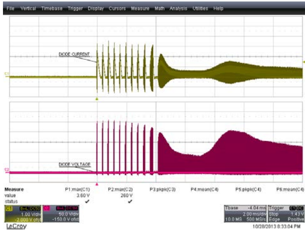
Figure 52 – 265 VAC, 50 Hz. Upper: I_{D7} , 1 A / div. Lower: V_{D7} , 50 V / div., 2 ms / div.
