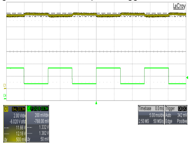
Figure 25 – Transient Response, 115 VAC, 50% \leftrightarrow 100% Step Load. Upper: V OUT , 2 V / div. Lower: I OUT , 1 A / div., 5 ms / div.
