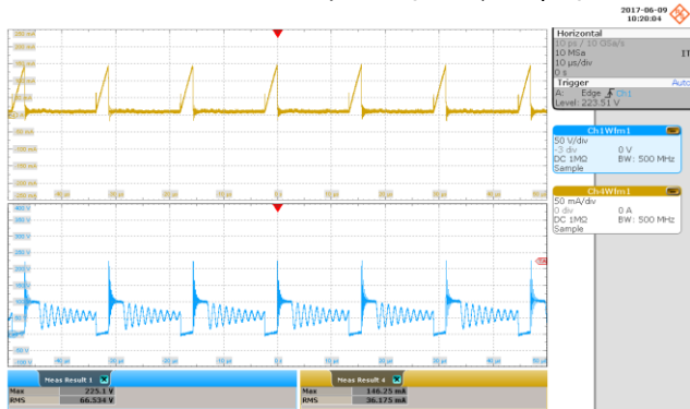
Figure 31 – 85 VAC Input. Condition: 3.8 V – 20 mA, 12 V – 20 mA. Upper: I_{DRAIN} , 50 mA / div. Lower: V_{DRAIN} , 50 V / div., 10 \mu s / div.
