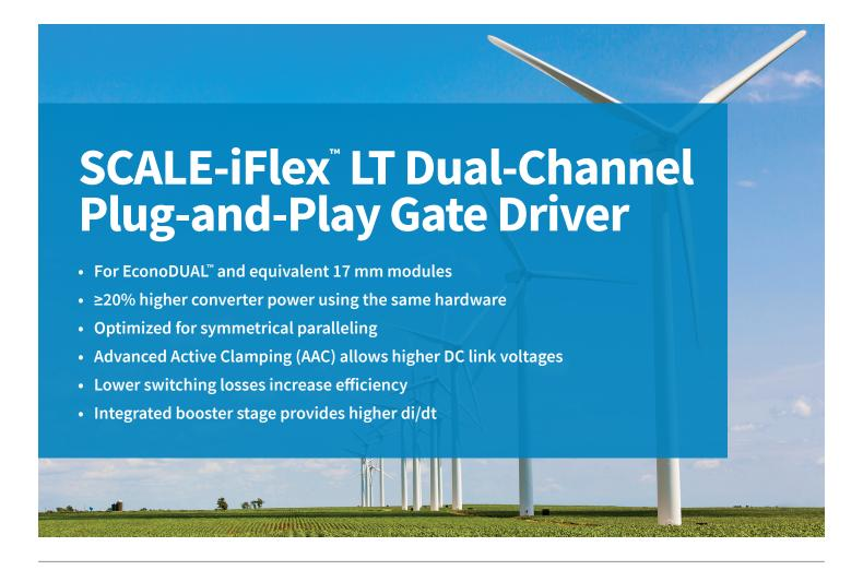
Isolated Master Control (IMC) and Module Adapted Gate Driver (MAG) for up to 1700 V Half-Bridge Power Modules
