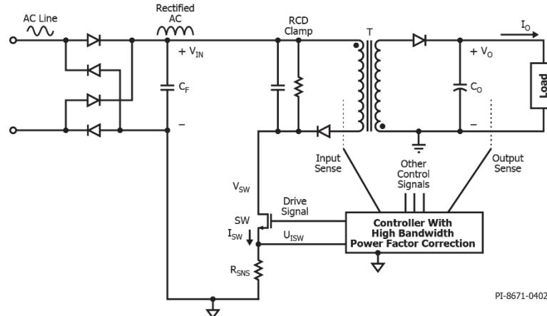
Figure 1. A flyback converter with HF process of switching current inside the controller and high bandwidth loop of power factor correction (PFC).
