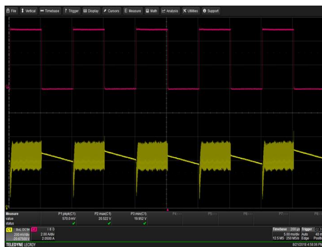
Figure 43 – Transient Response. 265 VAC, 20 V, 0 – 5 A Load Step. V_{MIN} : 19.952 V, V_{MAX} : 20.522 V. Upper: V_{OUT} , 0.2 V / div., 5 ms / div. Lower: I_{LOAD} , 1 A / div.
