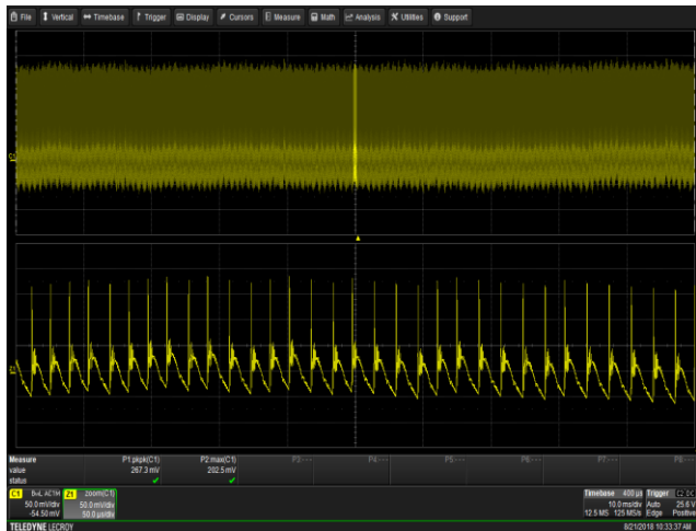
Figure 72 – Output Ripple. (PK-PK – 267.3 mV) 90 VAC Input, 20.0 V, 5 A Load. V_{OUT} , 50 mV / div., 10 ms / div.
