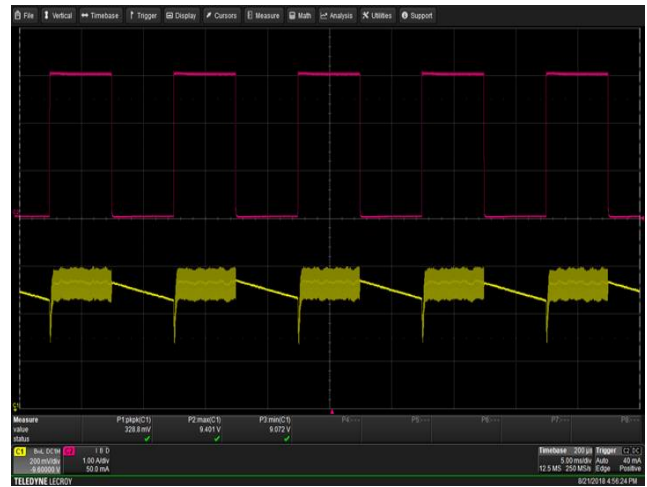
Figure 39 – Transient Response. 265 VAC, 9 V, 0 – 3 A Load Step. V_{MIN} : 9.072 V, V_{MAX} : 9.401 V. Upper: V_{OUT} , 0.2 V / div., 5 ms / div. Lower: I_{LOAD} , 1 A / div.
