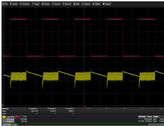
Figure 38 – Transient Response. 90 VAC, 9 V, 0 – 3 A Load Step. V_{MIN} : 9.009 V, V_{MAX} : 9.419 V. Upper: V_{OUT} , 0.2 V / div., 5 ms / div. Lower: I_{LOAD} , 1 A / div.
