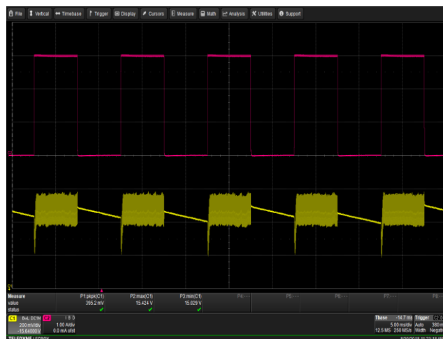
Figure 41 – Transient Response. 265 VAC, 15 V, 0 – 3 A Load Step. V_{MIN} : 15.029 V, V_{MAX} : 15.424 V. Upper: V_{OUT} , 0.2 V / div., 5 ms / div. Lower: I_{LOAD} , 1 A / div.
