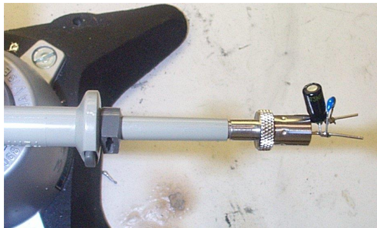
Figure 61 – Oscilloscope Probe with Probe Master ( www.probemaster.com ) 4987A BNC Adapter. (Modified with wires for ripple measurement, and two parallel decoupling capacitors added)
