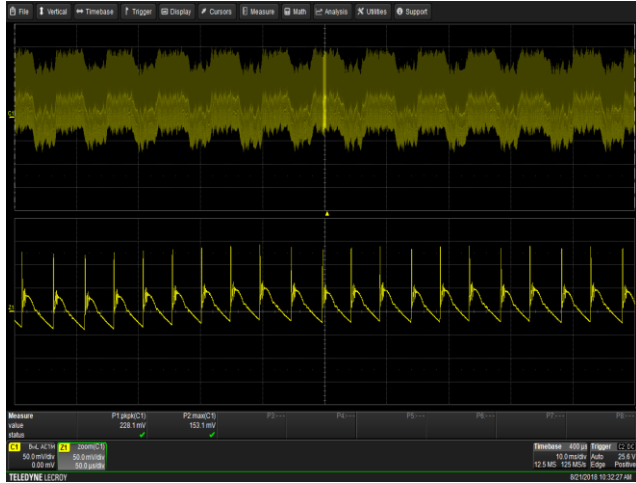
Figure 70 – Output Ripple. (PK-PK – 228.1 mV) 90 VAC Input, 15.0 V, 3 A Load. V_{OUT} , 90 mV / div., 10 ms / div.
