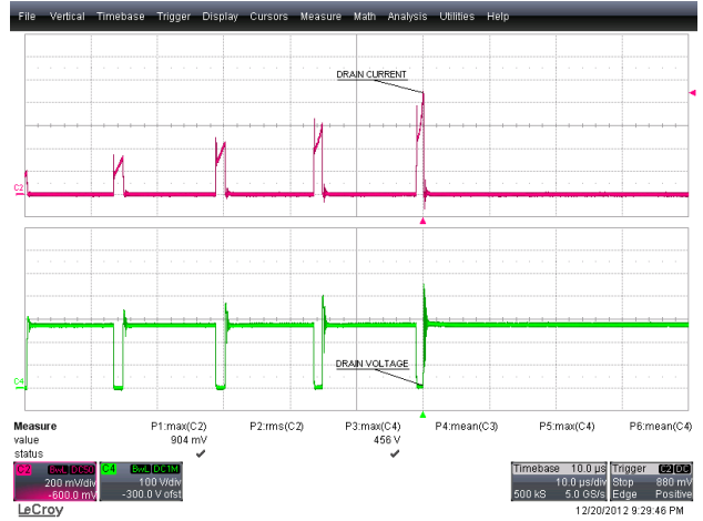
Figure 38 – 190 VAC, 50 Hz Start-up. Upper: I_{DRAIN} , 200 mA / div. Lower: V_{DRAIN} , 100 V, 10 \mu s / div.
