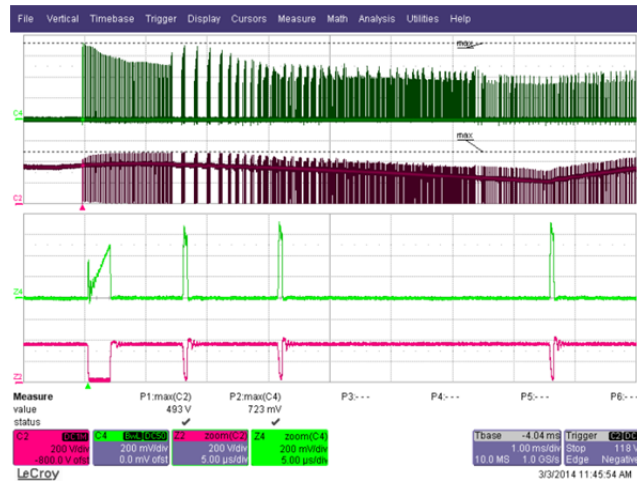
Figure 41 – 265 VAC Input and Maximum Load. Upper: I_{DRAIN} , 0.2 A / div. Lower: V_{DRAIN} , 200 V / div. Time Scale: 1 ms / div. Zoom Time Scale: 5 \mu s / div.
