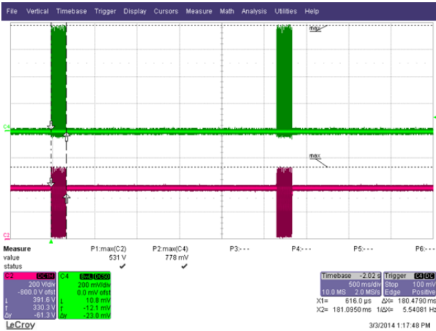
Figure 44 – 265 VAC Input, Full Load then Short. 180 ms Continuous Switching. Upper: I_{DRAIN} , 0.2 A / div. Lower: V_{DRAIN} , 200 V / div. Time Scale: 500 ms / div.
