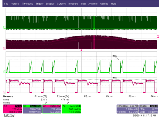
Figure 35 – 265 VAC, Full Load. Upper: I_{DRAIN} , 0.2 A / div. Lower: V_{DRAIN} , 200 V / div. Time Scale: 1 ms / div. Zoom Time Scale: 10 \mu s / div.
