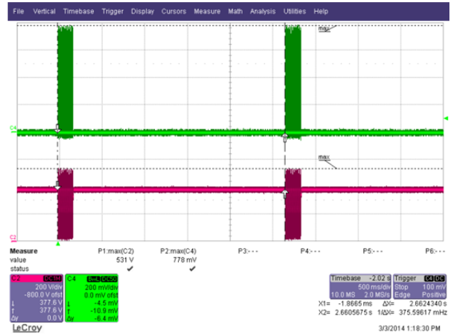
Figure 45 – 265 VAC Input, Full Load then Short. 2.5 s Off Time before Auto-restart. Upper: I_{DRAIN} , 0.2 A / div. Lower: V_{DRAIN} , 200 V / div. Time Scale: 500 ms / div.
