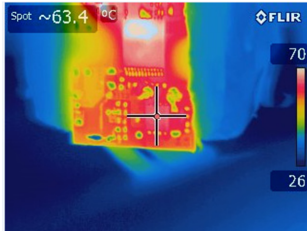
Figure 29 – Ambient = 28 °C. SR FET, Q3 = 63.4 °C.
