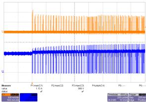
Figure 23 - Start-up Profile, 265 VAC, Full Load Upper: I<sub>DRAIN</sub>, 0.5 A / div. Lower:  $V_{DRAIN}$ , 200 V, 200  $\mu s$  / div.
