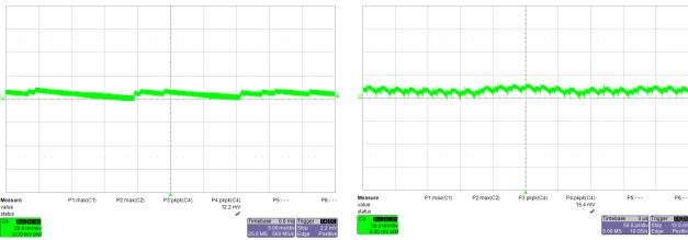
**Figure 38 –** Output Ripple, 265 VAC, No-Load 20 mV, 5 ms / div.
