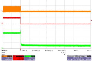
Figure 49 - Output Overvoltage (Open Loop),
