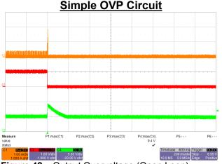
Figure 42 – Output Overvoltage (Open Loop), 90 VAC, No-Load
