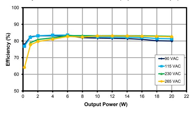
**Figure 9 –** Efficiency with 68  $\mu$ F Input Capacitor, Room Temperature.
