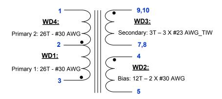
Figure 6 - Transformer Electrical Diagram.
