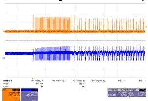
Figure 20 - Start-up Profile, 90 VAC, No-Load Upper:  $I_{DRAIN}$ , 0.5 A, 200  $\mu$ s / div.
