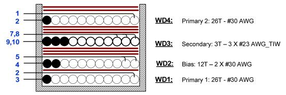
**Figure 7 –** Transformer Build Diagram.
