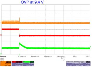
**Figure 44 –** Output Overvoltage (Open Loop), 265 VAC, No-Load
