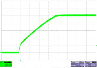
Figure 26– Output Voltage, 265 VAC, No-Load 1 V, 2 ms / div.
