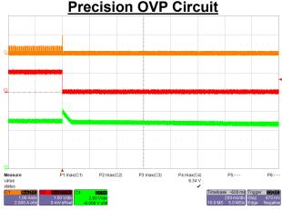
**Figure 43 –** Output Overvoltage (Open Loop), 90 VAC, No-Load
