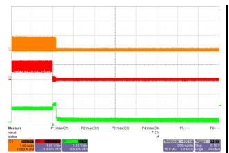
Figure 48 - Output Overvoltage (Open Loop),
