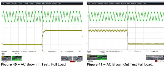
Figure 40 – AC Brown In Test., Full Load Upper: V<sub>IN</sub>, 100 V / div. Lower: V<sub>OUT</sub>, 2 V, 50 ms / div
