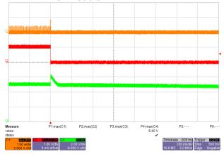
**Figure 45 –** Output Overvoltage (Open Loop), 265 VAC, No-Load
