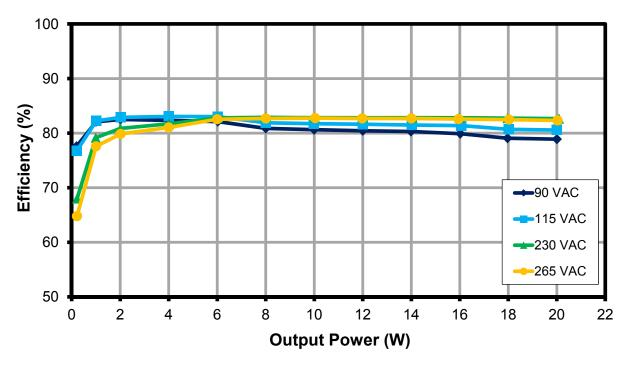
**Figure 8 –** Efficiency with 68 μF Input Capacitor and Thermistor In-Circuit, Room Temperature.
