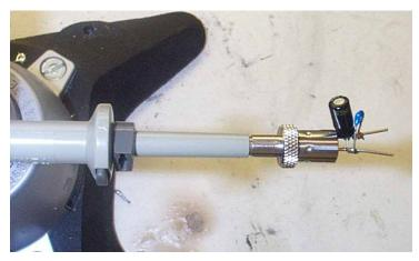
**Figure 31 –** Oscilloscope Probe with Probe Master (<u>www.probemaster.com</u>) 4987A BNC Adapter. (Modified with Wires for Ripple Measurement, and Two Parallel Decoupling Capacitors Added.)
