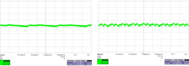
Figure 34 – Output Ripple, 115 VAC, No-Load 20 mV, 5 ms / div.
