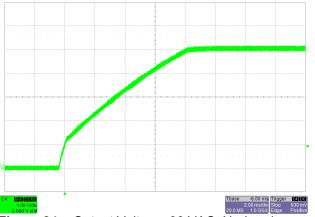
Figure 24 – Output Voltage, 90 VAC, No-Load 1 V, 2 ms / div.
