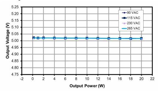
Figure 15 – Load Regulation, Room Temperature.
