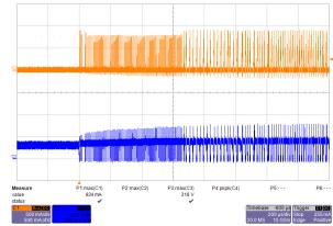
Figure 21 - Start-up Profile, 90 VAC, Full Load Upper:  $I_{DRAIN}$ , 0.5 A, 200  $\mu s$  / div.
