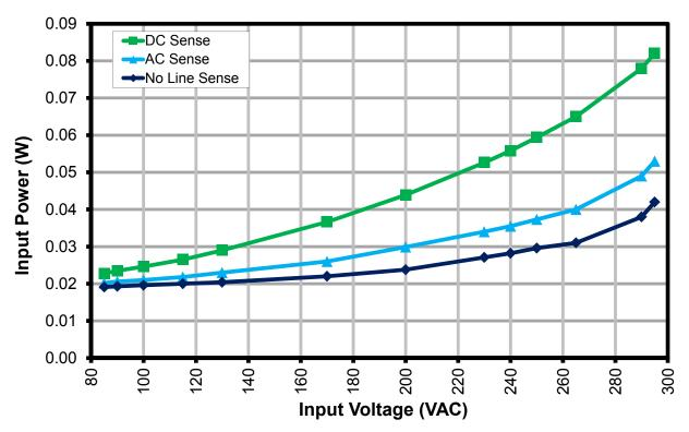
Figure 12 – Input Power at No-Load.
