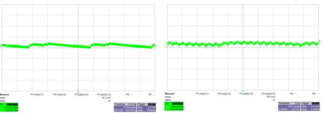
Figure 36 – Output Ripple, 230 VAC, No-Load 20 mV, 5 ms / div.
