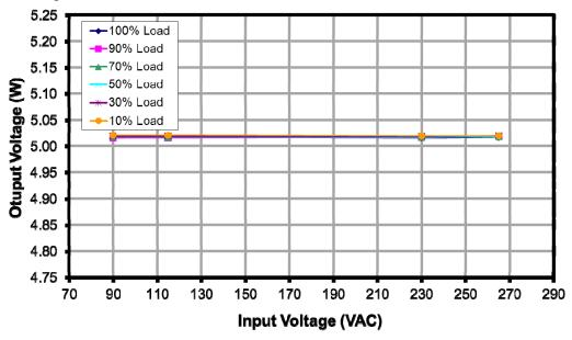
Figure 16 – Line Regulation, Room Temperature.
