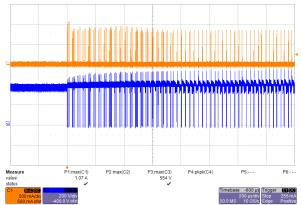
Figure 22 - Start-up Profile, 265 VAC, No-Load. Upper: I<sub>DRAIN</sub>, 0.5 A / div.
