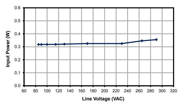
Figure 13 – Input Power at 250 mW Load, Room Temperature.
