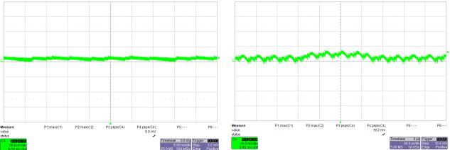
Figure 32 – Output Ripple, 85 VAC, No-Load 20 mV, 5 ms / div.
