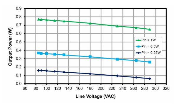
Figure 14 – Output Power at 0.25 W, 0.5 W and 1 W of Input Power, Room Temperature.
