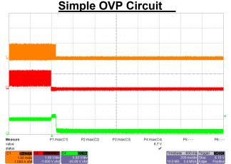
Figure 46 - Output Overvoltage (Open Loop),
