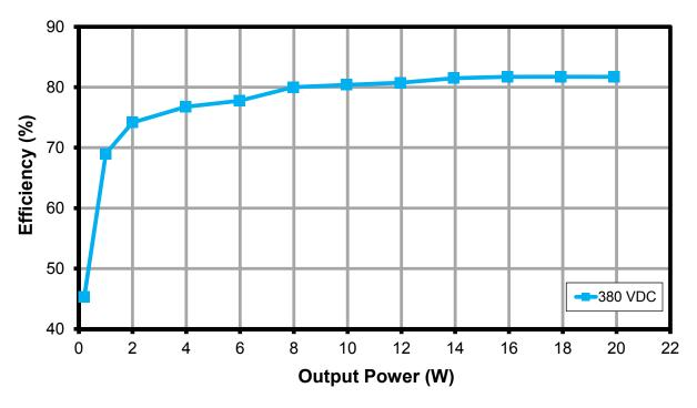
Figure 10 – Efficiency with 220  $\mu$ F Input Capacitor, Room Temperature.
