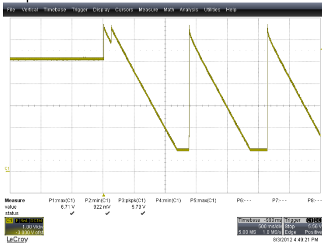
Figure 57 – Output OVP, 265 VAC, Standby Load. V_{OUT} , 5 V, 1 V, 500 ms / div.
